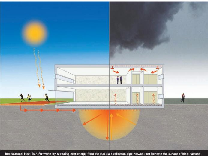
Interseasonal Heat Transfer works by capturing heat energy from the sun via a collection pipe network just beneath the surface of black tarmac roads (or car parks or school playgrounds). It then stores the energy in computer-controlled thermal banks in the ground under the foundation of buildings, and releases it to heat the buildings in winter via heat pumps linked to underfloor heating.
