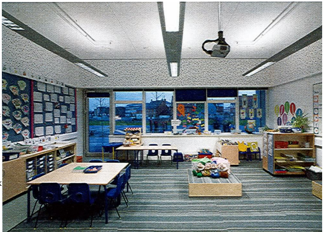
Right/above Strategically placed rooflights allow daylight to flood into the centre of the building, minimizing the need for artificial lighting of deep-plan spaces.
