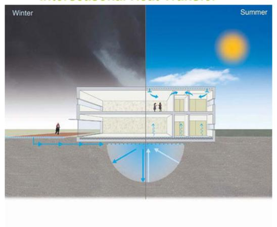
IHT captures coolth in winter stores it in ThermalBanks releases it in summer to provide cooling without the horrendous cost of air conditioning
