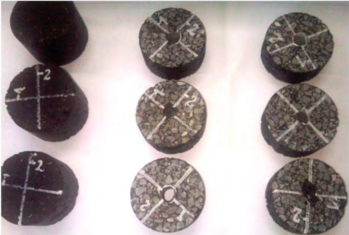
Fig. 58. SMA samples before the ITS test. The left row - samples without a tube, middle - RB1,2,6 samples compacted with a bolt, on the - right RBB1,2,7 samples compacted without a bolt.
