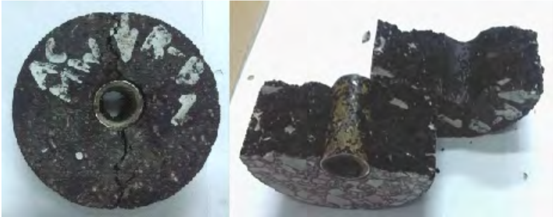
Fig. 56. RB1 Sample after testing – cracks along load axis and fracture samples without tubes after ITS tests.
