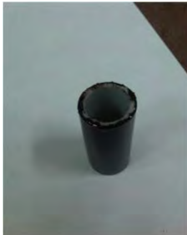
Fig. 52. Tube preparation (overlying with binder) intended for being placed in the sample.
