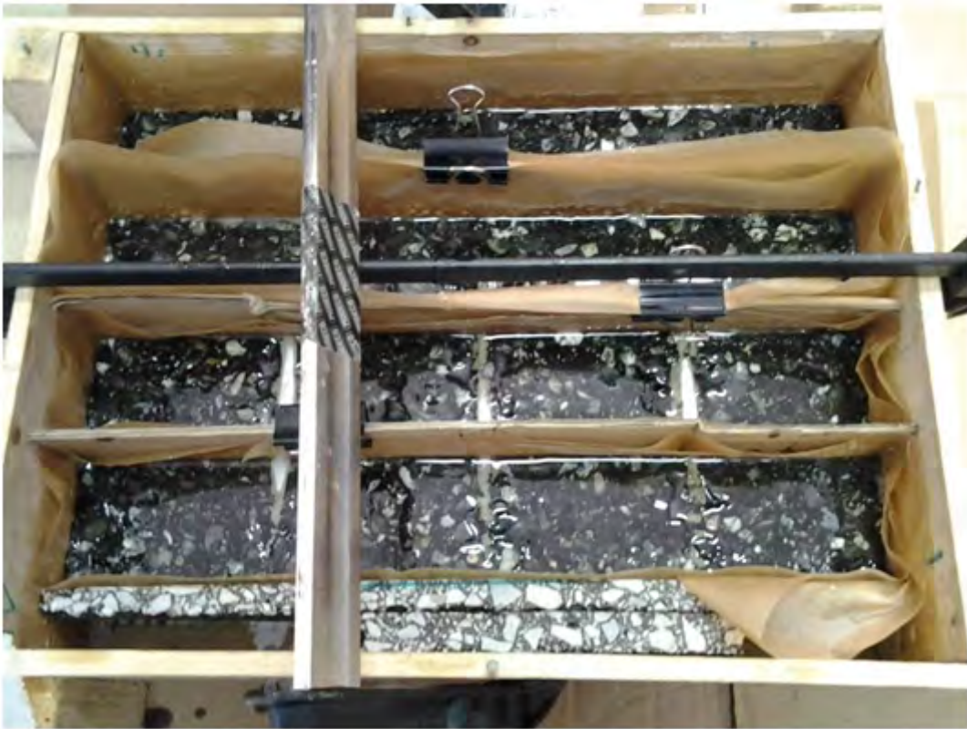
Fig. 83. Beams coated with resin – prepared for applying the aggregate.
