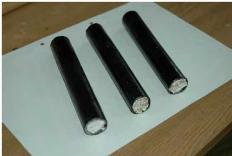
Fig. 80. Tubes coated with binder before installation in the mineral-asphalt mix.
