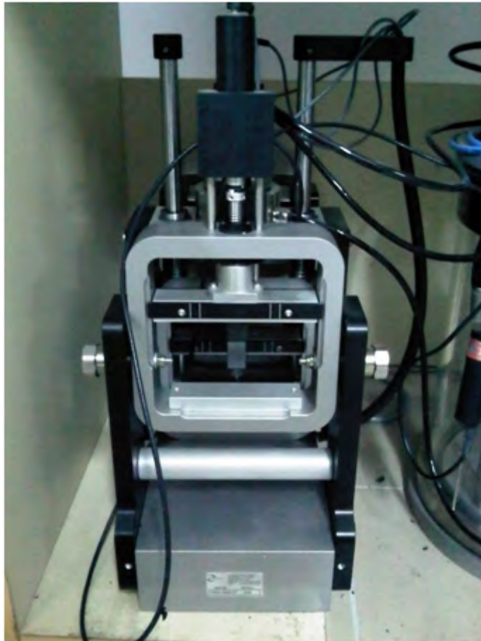
Fig. 82. Addition to the test using four point bending method.
