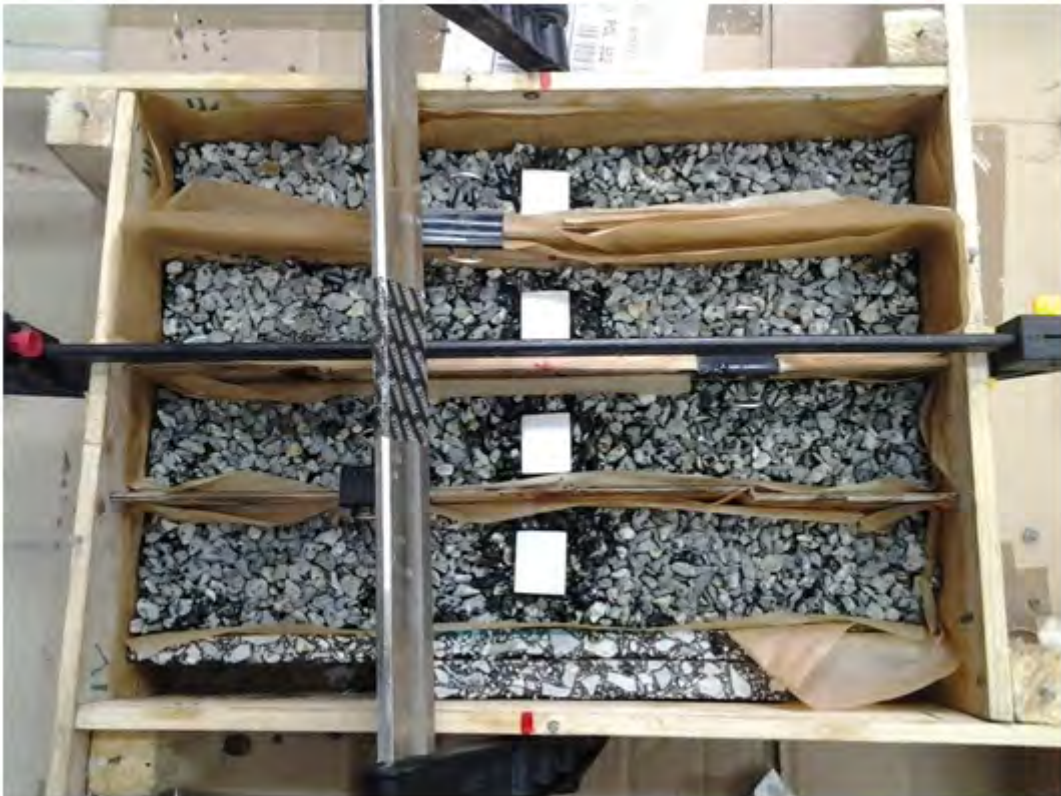
Fig. 84. Beams with 2 layers of aggregate on resin.
