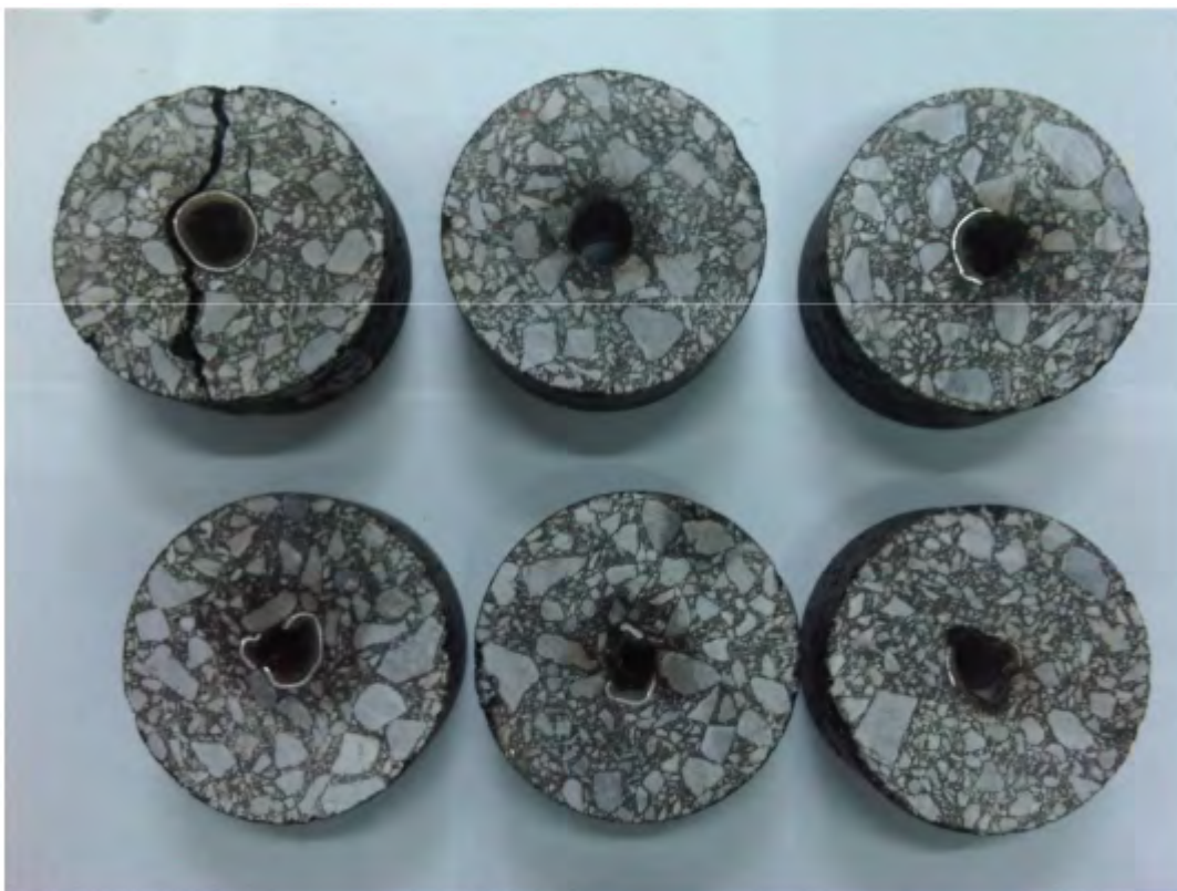
Fig. 57. Visual appearance of the rear part of asphalt concrete samples after ITS tests. The upper row is RB1-3 samples, the lower - RBB1-3.
