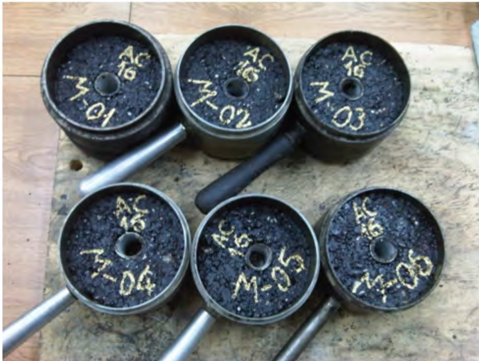
Fig. 61. Roll samples AC16W for testing frost resistance after formation the Marshall tamper.
