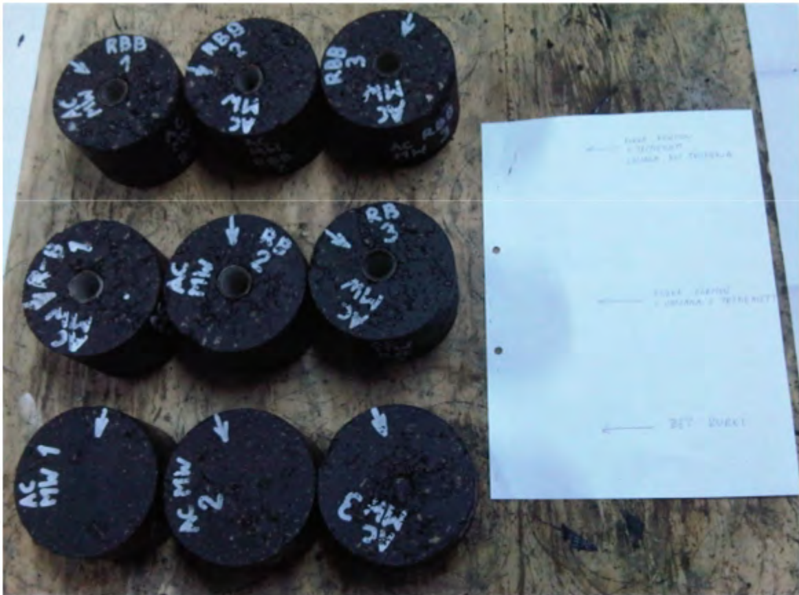
Fig. 53. Samples of asphalt concrete prepared for ITS tests.
