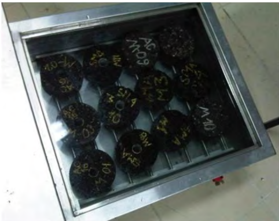
Fig. 62. A batch of samples for frost resistance testing during soaking in water with the temperature of 40 and 60°C.
