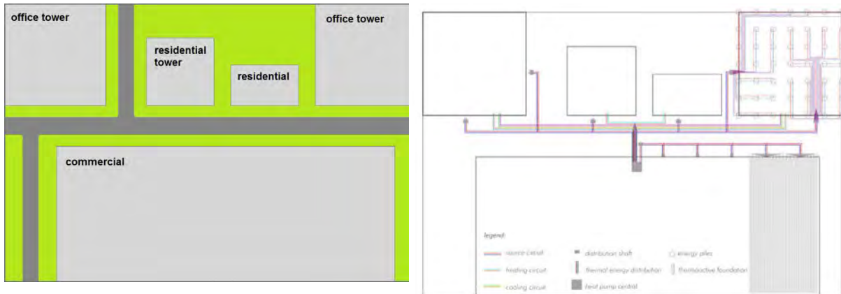
Fig. 4. District lay-out (left) and piping network between buildings when using a central heat pump (right). The energy system includes an energy pile system underneath the office towers and a thermoactive plate foundation under the commercial building.
