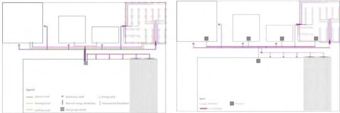
Fig. 39. piping network alternatives, left: central heat pump, right: generation at building level.
