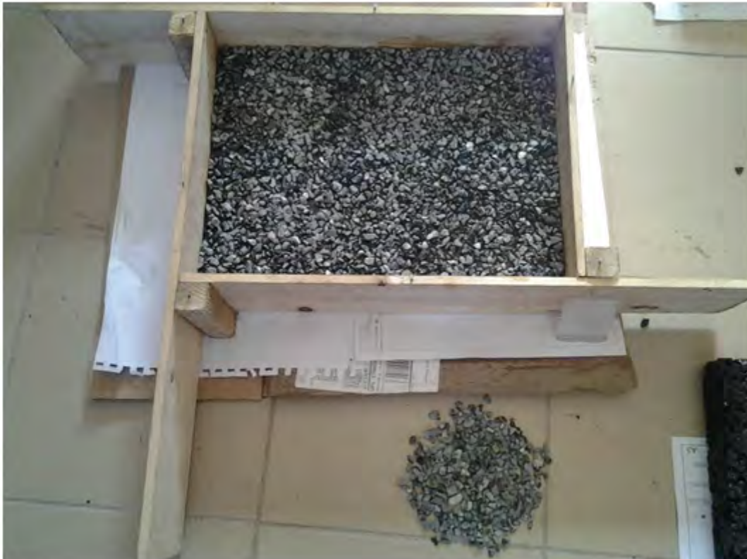
Fig. 65. Sample 1 after laying the 1st aggregate layer on resin.
